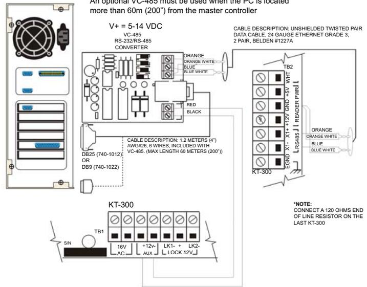
\*NOTE: CONNECT A 120 OHMS END OF LINE RESISTOR ON THE LAST KT-300
